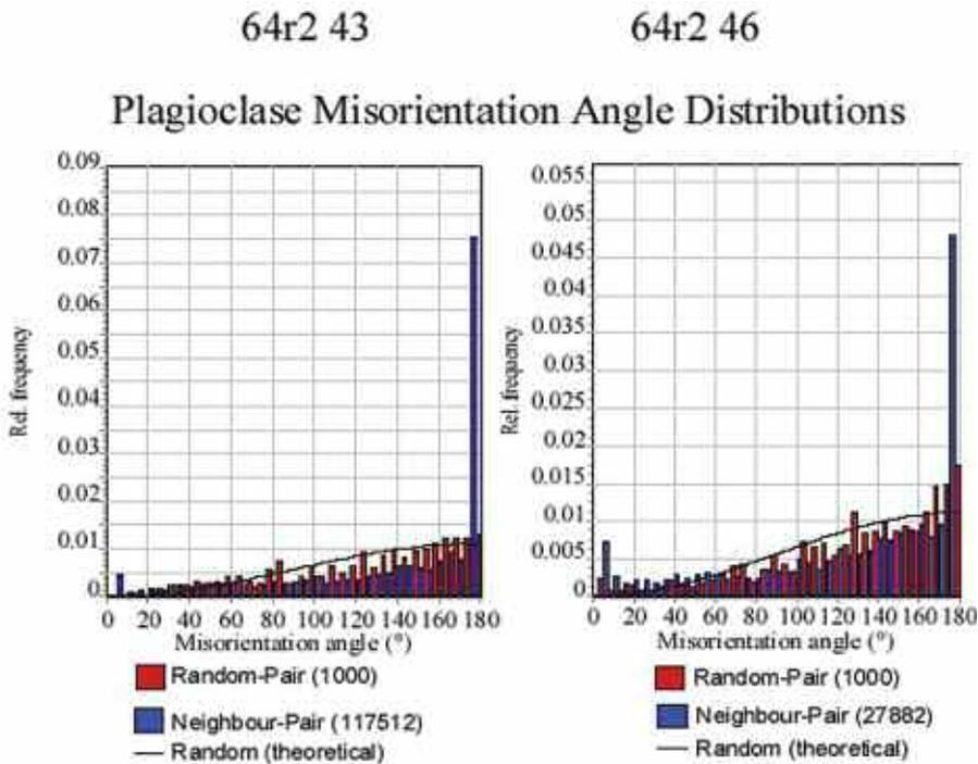
Figure 6. Misorientation angle distributions for 64r2 43 and 64r2 46 are plotted as frequency histograms for neighbour-pairs and random-pairs. The black line represents the theoretical random distribution. 64r2 43, random-pairs 1000 data points and neighbour-pairs 117512 data points. 64r2 46, random-pairs 1000 data points and neighbour-pairs 27882 data points.
