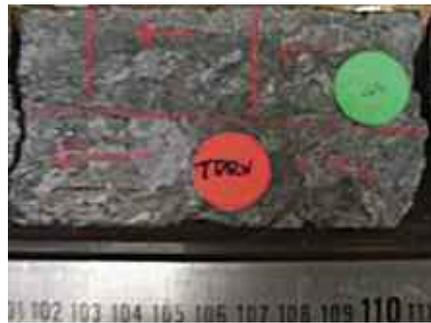
Figure 2. Photograph of core 270r3 section 101 to 111cm (from the top of the core). The piece of the core exhibits red markings which show the boundaries of each sample. So the core will be cut into one half slab (red sticker saying Toru) and two thin section billets (one for me and one for AD). The arrows mark the orientation of core up.
