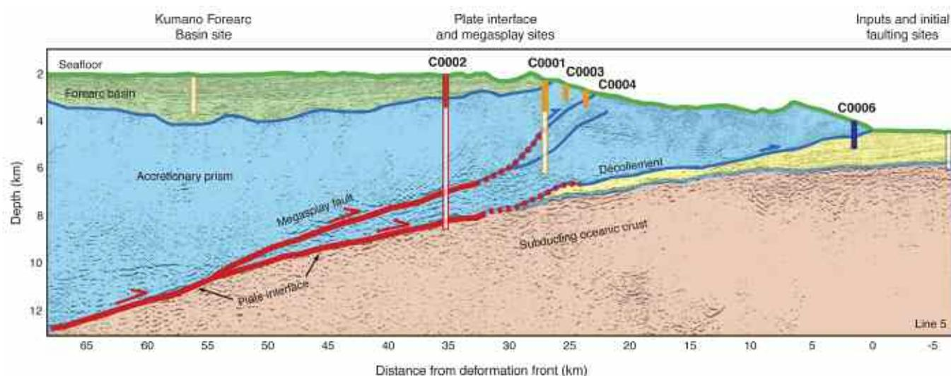
Figure 2. A seismic profile section showing the location and depth of the five sites across the subduction zone during Expedition 314, and the planned future riser and non-riser sites. Location shown on Figure 1 (Line 5).
