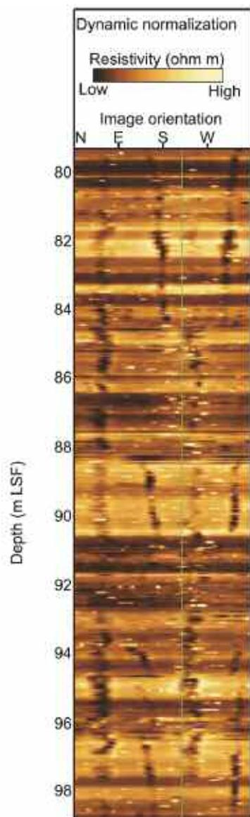
Figure 5. Resistivity image at Site C0001 showing borehole breakouts (vertical conductive lines at NE and SW) and drilling-induced tensile fractures (near-vertical conductive lines at SE and NW) indicating shortening at  $\sim 335^\circ$  or perpendicular to the margin and plate boundary.
